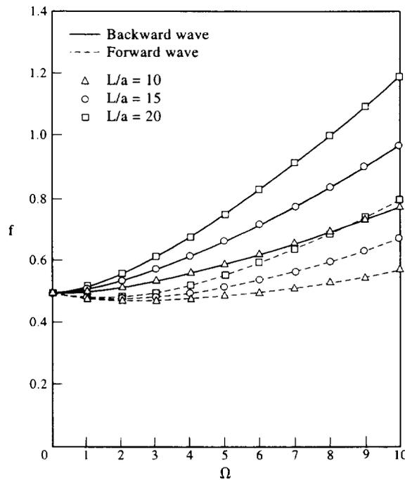
Fig. 8. Relationship between the frequency parameter  $f$  and rotating speed  $\Omega$  (rps = revolutions per second or Hz) at various non-dimensional geometric coefficient  $L/a$  ( $m = 1, n = 2, \alpha = 45^\circ, \mu = 0.3, h/a = 0.02$ ).
