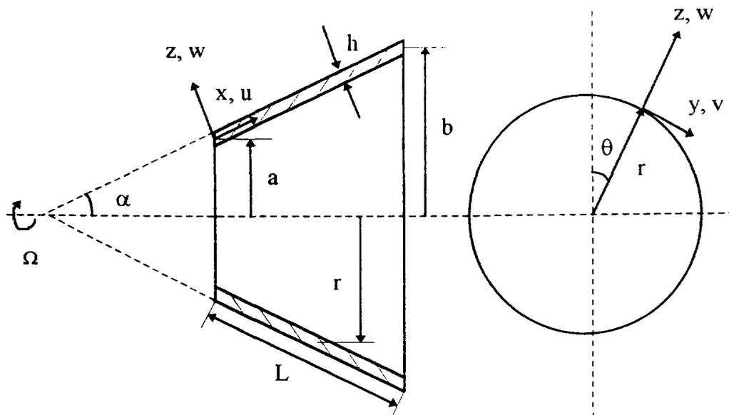
Fig. 1. The geometry of a truncated circular conical shell.
