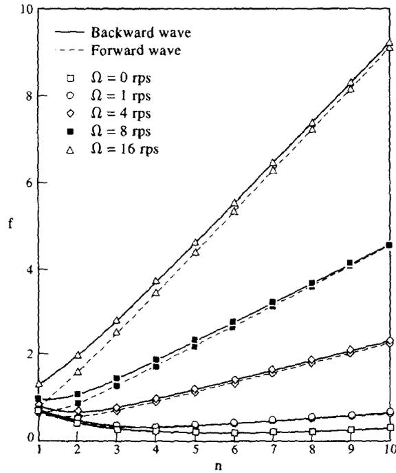
Fig. 6. Relationship between the frequency parameter  $f$  and circumferential wave number  $n$  at various rotating speeds for cone angle  $\alpha = 60^\circ$  ( $m = 1, \mu = 0.3, h/a = 0.02, L/a = 20$ ).
