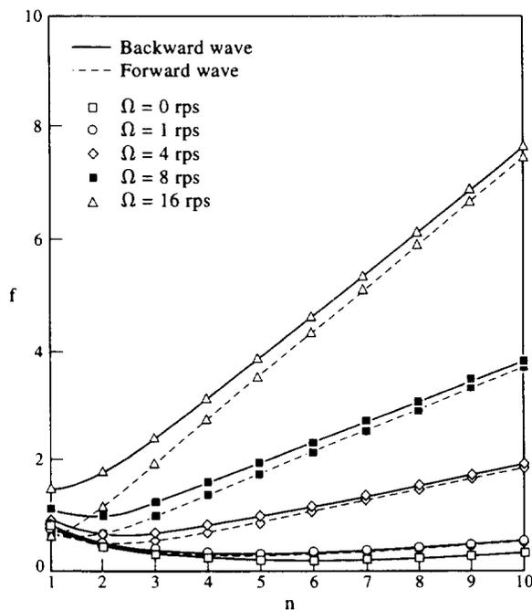
Fig. 5. Relationship between the frequency parameter  $f$  and circumferential wave number  $n$  at various rotating speeds for cone angle  $\alpha = 45$  ( $m = 1, \mu = 0.3, h/a = 0.02, L/a = 20$ ).
