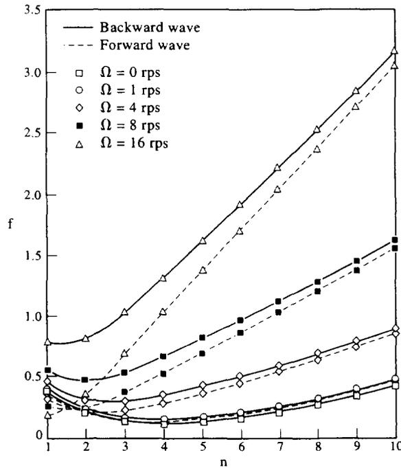
Fig. 3. Relationship between the frequency parameter  $f$  and circumferential wave number  $n$  at various rotating speeds for cone angle  $\alpha = 15^\circ$  ( $m = 1, \mu = 0.3, h/a = 0.02, L/a = 20$ ).
