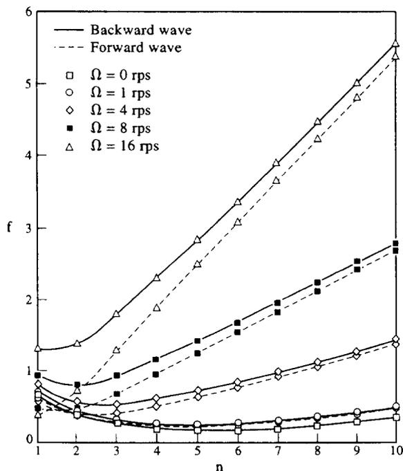
Fig. 4. Relationship between the frequency parameter  $f$  and circumferential wave number  $n$  at various rotating speeds for cone angle  $\alpha = 30$  ( $m = 1, \mu = 0.3, h/a = 0.02, L/a = 20$ ).
