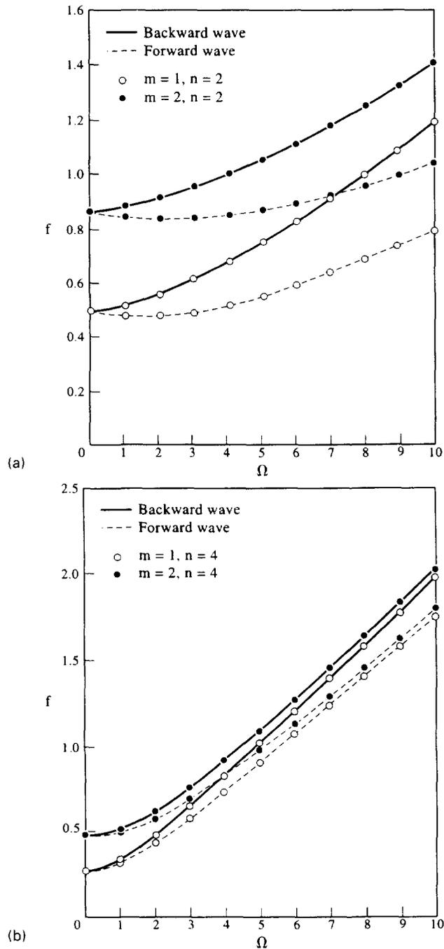
Fig. 9. Relationship between the frequency parameter  $f$  at various modes of free vibration and rotating speed  $\Omega$  ( $\mu = 0.3$ ,  $\alpha = 45^\circ$ ,  $h/a = 0.02$ ,  $L/a = 20$ ).
