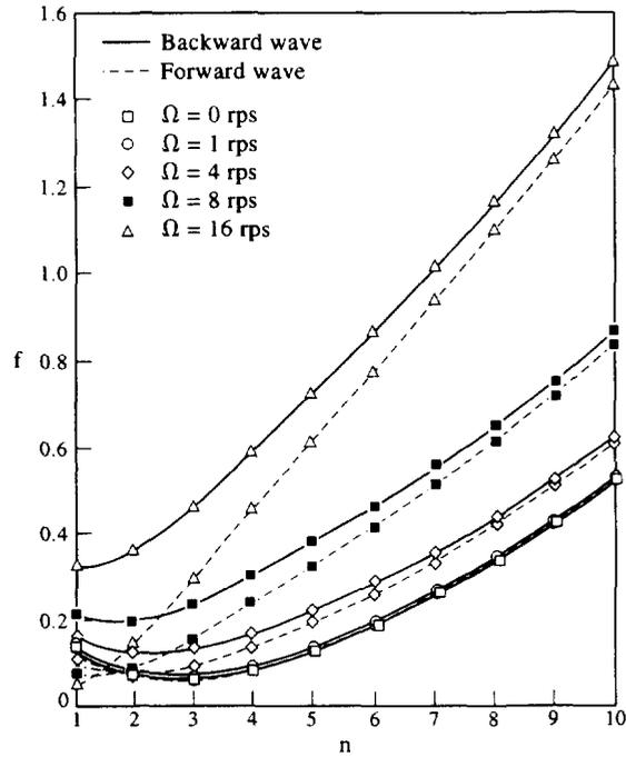
Fig. 2. Relationship between the frequency parameter  $f$  and circumferential wave number  $n$  at various rotating speeds for cone angle  $\alpha = 5^\circ$  ( $m = 1, \mu = 0.3, h/a = 0.02, L/a = 20$ ).
