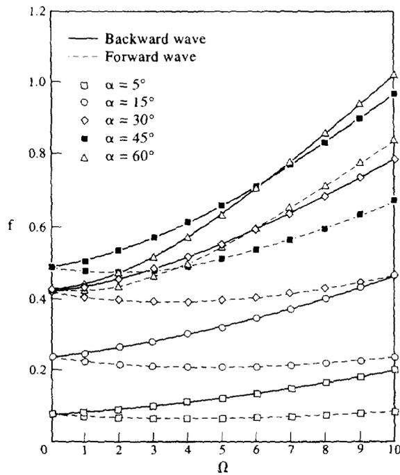
Fig. 7. Relationship between the frequency parameter  $f$  and rotating speed  $\Omega$  (rps = revolutions per second or Hz) at various cone angle  $\alpha$  ( $m = 1, n = 2, \mu = 0.3, h/a = 0.01, L/a = 15$ ).
